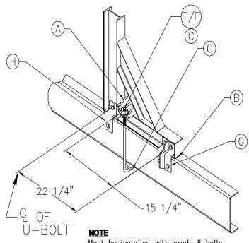
Must be installed with grade 8 bolts, nuts and hardened washers. (not included)
