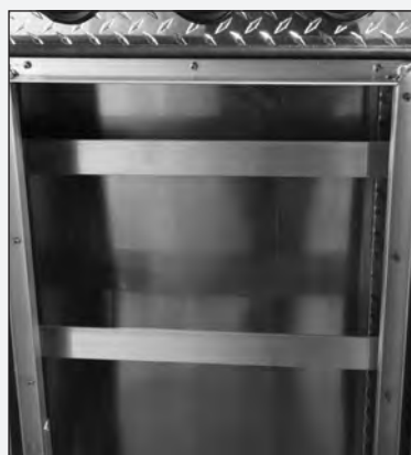
Chain hangers in each side compartment
