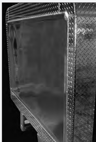
No rear Beams. You can get the unit closer to the cab than a normal CR.
